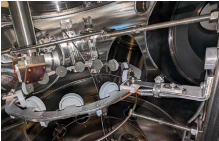
B-dot probe in-vessel in the WHAM device
